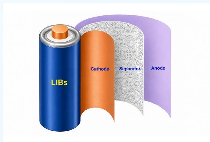
Figure 2: Illustration of a jelly-roll style battery.
