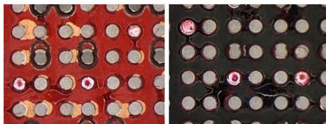
Figure 8: Solder joints on the board (left) and component (right) sides of the PCB, are marked by red dye, indicating head-in-pillow defects.
