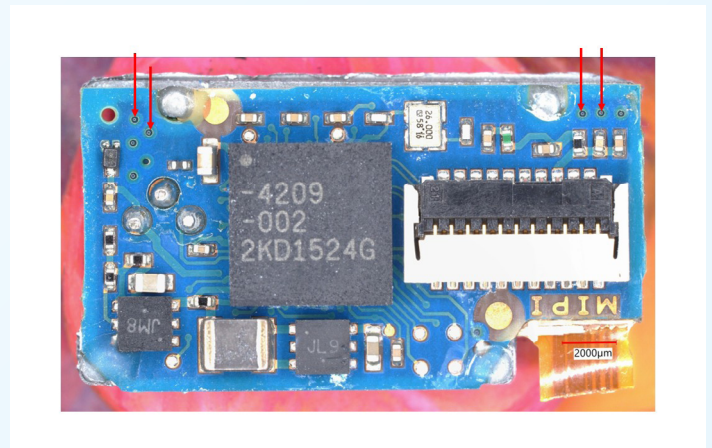
Figure 4: Optical image of PCB with suspect regions indicated for electrical testing.
