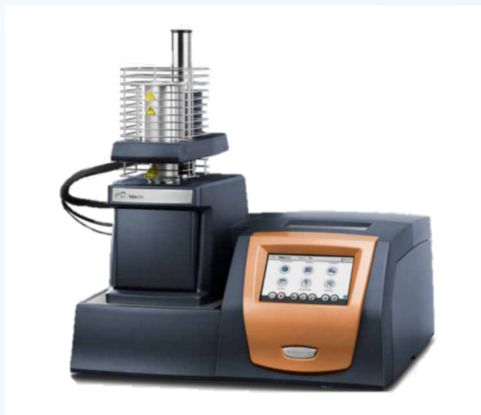
Figure 5: At Covalent, we use a TA Instruments Discovery TMA 450 EM.
